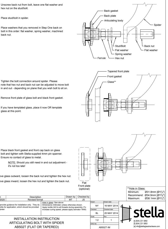
Step 7 Place black front gasket and front cap back on glass bolt and tighten with Stella-supplied 4mm pin spanner.
