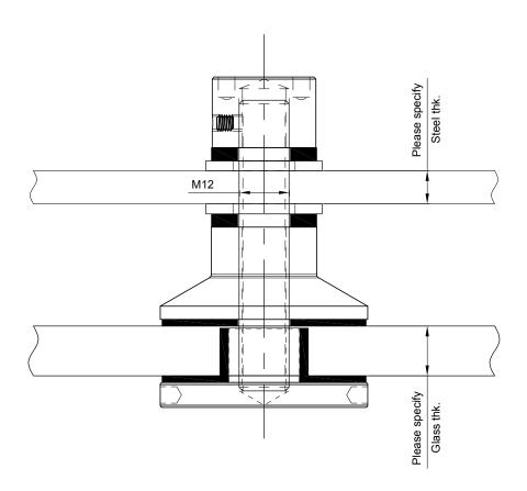
Hole in glass min. Ø22.2mm [Ø $^{7}$ / $_{8}$ "] recommend Ø25.4mm [Ø1"]
