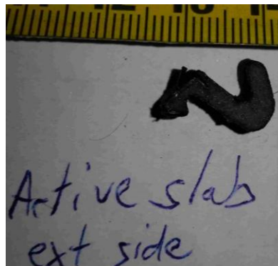
Figure 32 – Vinyl wrapped foam filled weather-stripping on active slab, exterior side.
