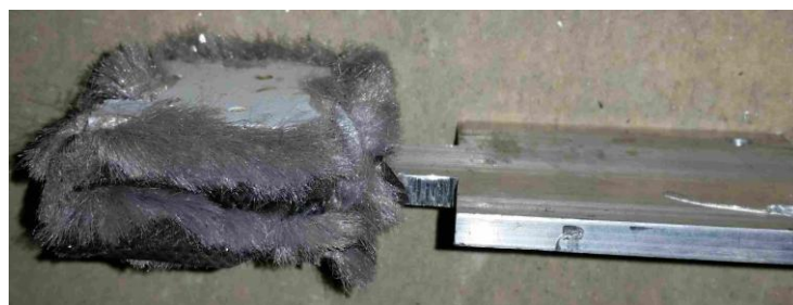
Figure 16 – Weather-stripping around aluminum profile
