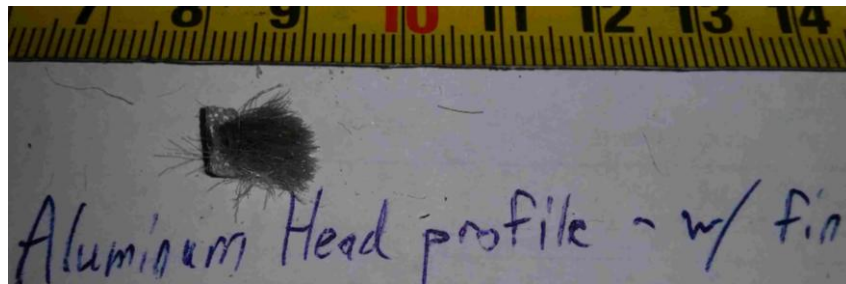
Figure 27 – Head track pile weather-stripping with center fin
