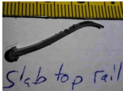
Figure 25 – Rubber fin seal used on the sill, head, top rail of sash and fixed slab mullion side
