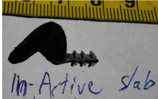
Figure 33 – Foam weather-stripping on in-active slab locking stile
