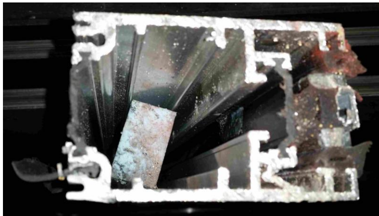
Figure 7 – Common rail/stile sash profile
