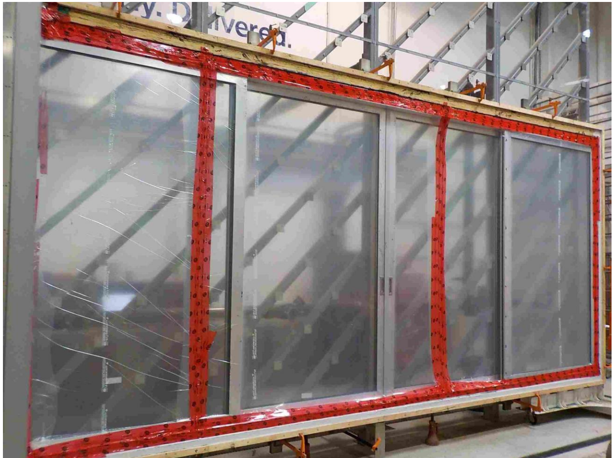
Figure 1 - XXXO Sliding Door – Exterior side *Note – Picture taken during air leakage test, with poly bag in place.
