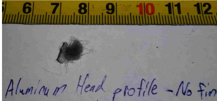
Figure 26 – Head track pile weather-stripping
