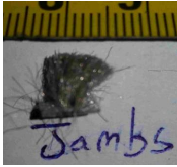
Figure 23 – Jamb pile weather-stripping
